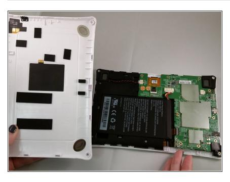
After the back case is loosened, remove it from the device to change or access the battery.
