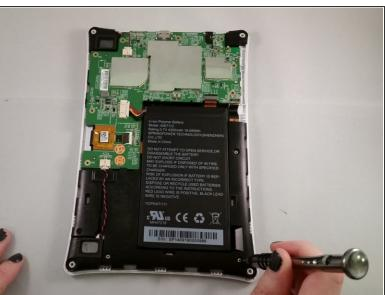
Unscrew the circuit board from the motherboard by using a Phillips #0 screwdriver to unscrew the ten 4mm screws in a counter-clockwise rotation.
