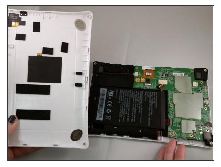
After the back case is loosened, remove it from the device to change or access the battery.
