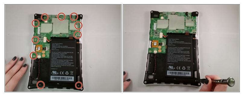
Unscrew the circuit board from the motherboard by using a Phillips #0 screwdriver to unscrew the 4mm screws in a counter-clockwise rotation.
