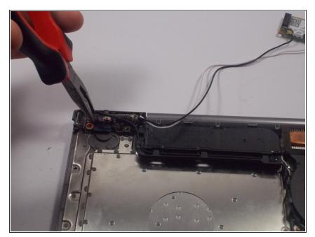
Using a pair of long-nose pliers, grab onto the hinge in the upper lefthand corner of the screen and pull it upward, similarly to how you open a laptop.
