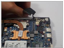
Using the black tab on top of the IDE plug, carefully lift the plug vertically upward until it is disengaged from the socket. This piece is attached to the base by a black wire, and can be left here for the duration of the replacement.
