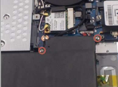
On each side of the portion that is jutting out, there is one, silver 1.5 mm screw. Using the Phillips #00 screwdriver, remove these two screws.
