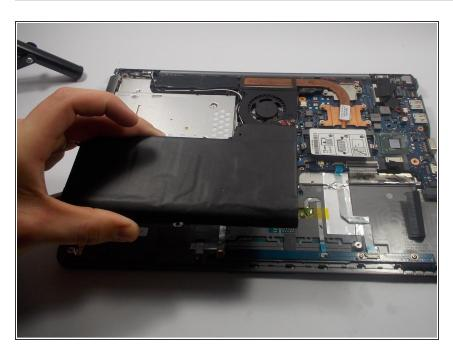
Using your dominant hand, carefully lift the battery vertically out of place, making sure to handle with care and to not bump any other parts of the computer. To reassemble your device, follow these instructions in reverse order.
