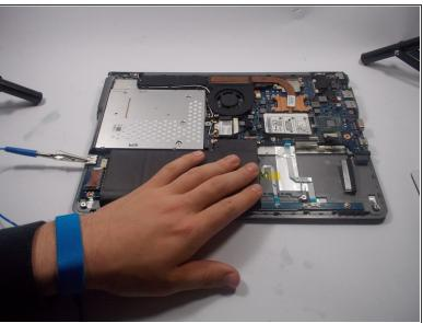
All steps following the removal of the back cover should be completed while wearing an Anti static bracelet. This prevents ESD (electrostatic discharge). ESD can damage nearly every part on the inside of your computer.
