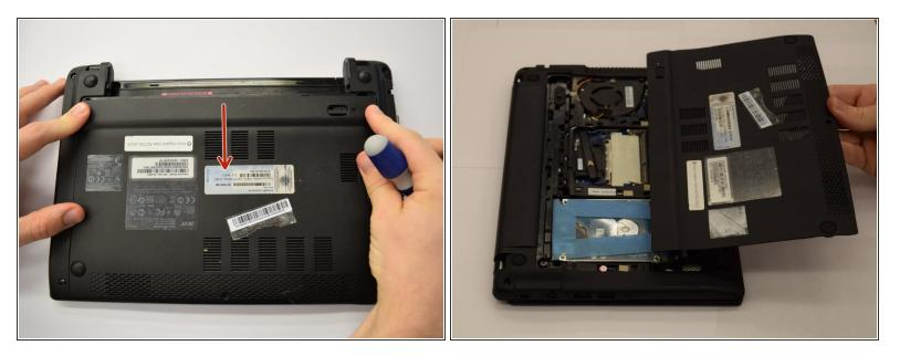
• Slide the back plate downward to remove it from the laptop.
