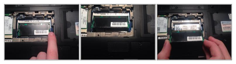
• Remove the RAM. Push on the two tabs holding the module in the laptop and lift the module by the edges.
