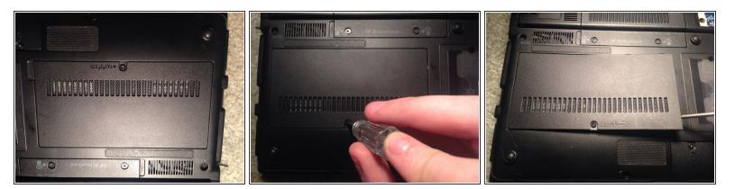
• Remove the RAM/Wireless card cover to access the RAM.
