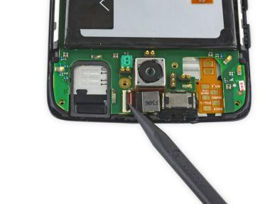
Use the pointed end of a spudger to flip up the black retaining flap of the front facing camera's ZIF connector.
