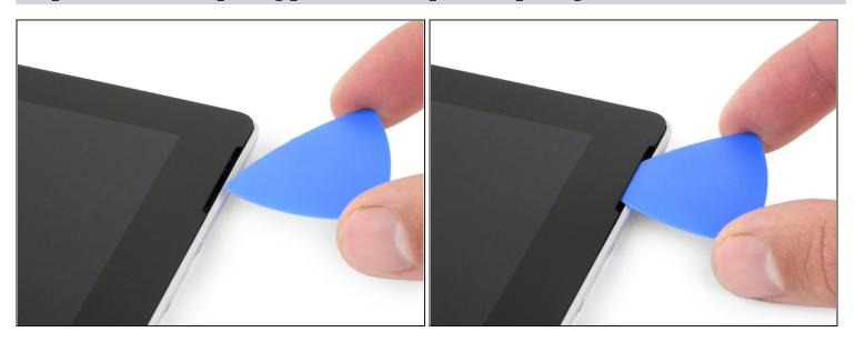
• Insert an opening pick into the top-right speaker cutout on the screen and slide the pick between the glass and speaker grille.
