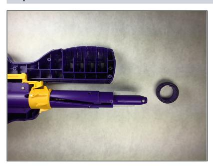
• Slide the rubber ring off of the barrel and set it aside.
