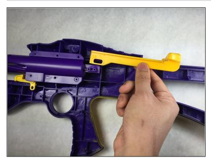
• Lift the yellow lever bar out of place and set aside.
