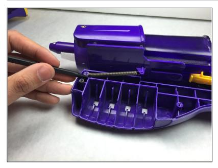
Using a spudger, unhook the barrel shield's spring from the right half of the toy gun. One side should still be connected to the shield barrel shield.
