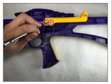
Use a Phillips #1 screwdriver to unscrew the two 12 mm long washer head screws from the yellow loading bar lever.
