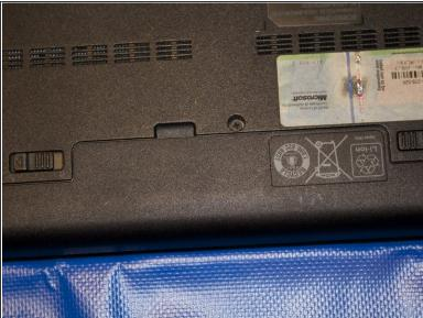
Place the battery and lock it into place
