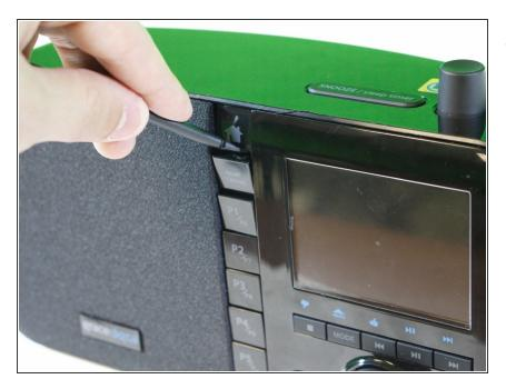
Remove the selection keys from the top using a plastic spudger.
