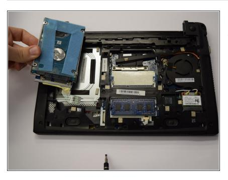
Remove the hard drive by pulling it straight out. To reassemble your device, follow these instructions in reverse order.
