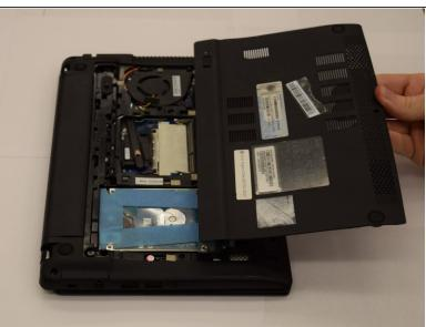
Slide the back plate downward to remove it from the laptop.
