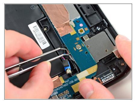
Pull the vibrator motor connector straight away from its socket on the USB connector board.
