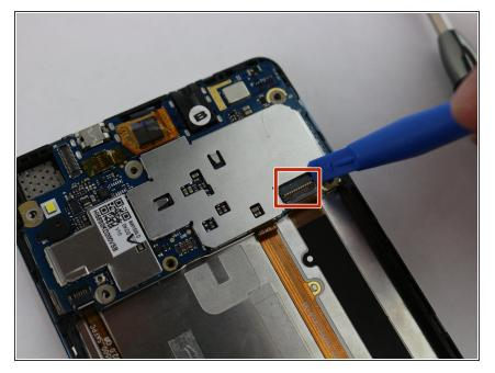
Lift the black tab on the zero insert force connector on the lower right side of the motherboard using a small blue plastic opening tool.
