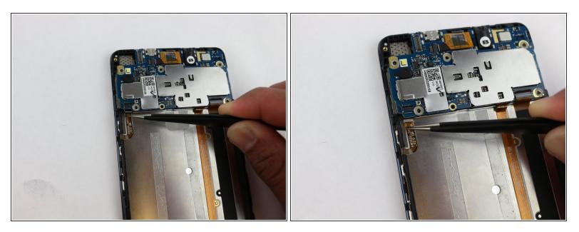
• Use a fine nose pair of tweezers to pull the ribbon cable from the zero insert force connector with little force to remove the contact connecter from the motherboard.
