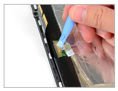
• Use the edge of a plastic opening tool to peel up the self-adhesive pull tab stuck to the display data cable.
