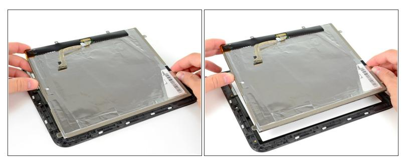
• Lift up the LCD assembly and remove it from the front panel.
