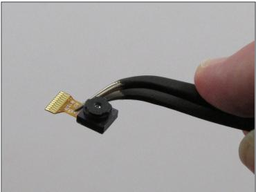
• Using precision <u>tweezers</u>, gently pull the camera off the motherboard.
