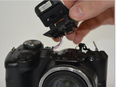
Firmly grasp the flash bulb lid and remove the lid from the camera.
