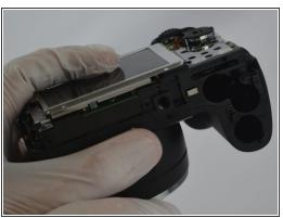
Once the back plate is removed twist the battery cover clockwise and it should easily dislodge.
