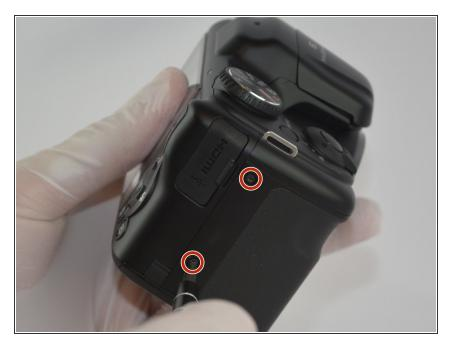
Use your Philips Head Screwdriver to remove the M3 x 4mm screws from the right side of the device as indicated by the pictures.
