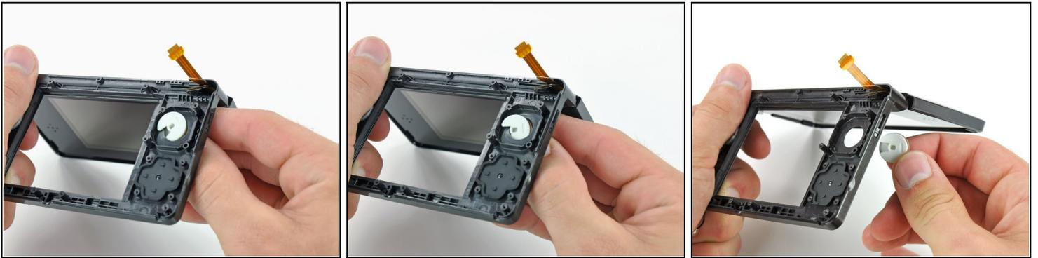
ⓘ Open the 3DS and hold it so that the bottom of the buttons are facing upward.
