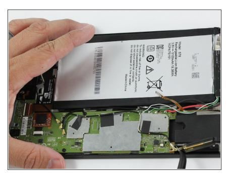
Using the angled tweezers, begin removing the antenna from the device.
