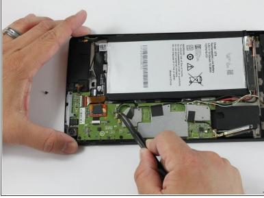
• Using the tweezers or your fingers lift the remaining black wires from the motherboard.
