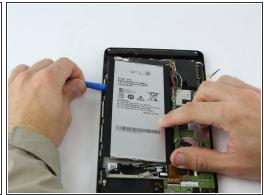
Once you have the blue plastic opening tool underneath the battery, work the tool around the edges of the battery similar to the technique used for the back panel.
