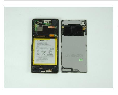
Remove the back cover by pulling it from the chassis. it is flexible and can be bent, be careful.
