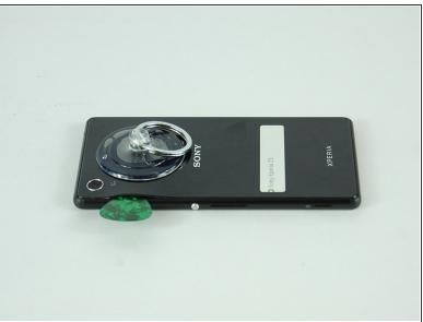
• While Pulling on the suction cup, slide a thin plastic spacer (guitar picks work well) between the back cover and the phone. Slide it around the edges to break the adhesive seal. Be careful, but don't be afraid to use some force. You should hear a sticky breaking sound.
