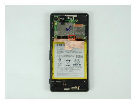
Unhook the battery connector carefully. It is possible to damage the battery if too much force is used.
