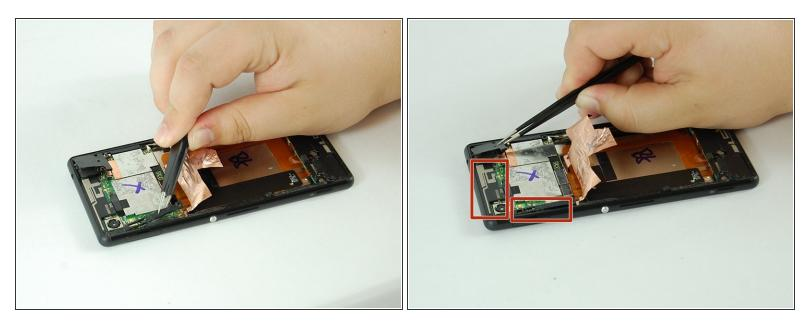
Remove three pieces of the securing bracket using tweezers
