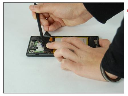
Remove copper plated tape and any other securing adhesive with a nylon spudger. Remove carefully, as it has the potential or tear if too much force is used.
