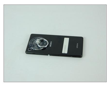
Attach a suction cup to the back of the M4 Aqua by carefully pushing down on it near the top of the phone.
