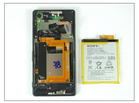
Remove the battery once all of the adhesive is broken, and the connector is unplugged.
