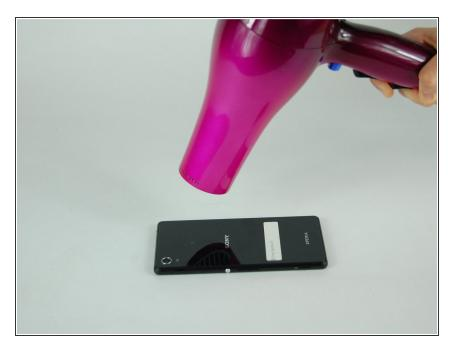
Place the phone face-down, and use a heat gun or hair dryer to evenly heat the back surface until to soften the adhesive.
