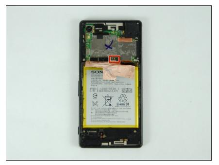
Unhook the battery connector carefully. It is possible to damage the battery if too much force is used.
