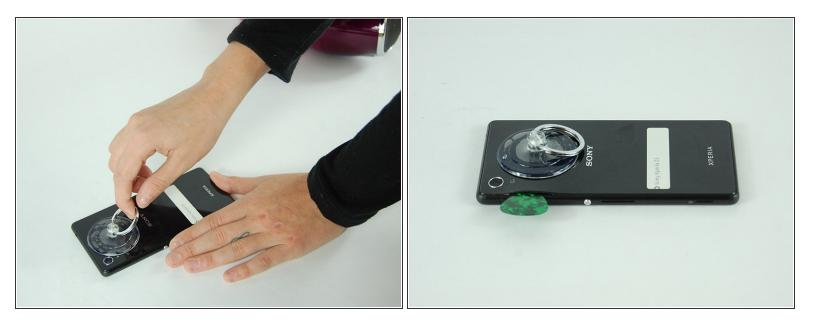
• While Pulling on the suction cup, slide a thin plastic spacer (guitar picks work well) between the back cover and the phone. Slide it around the edges to break the adhesive seal. Be careful, but don't be afraid to use some force. You should hear a sticky breaking sound.
