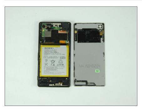
Remove the back cover by pulling it from the chassis. it is flexible and can be bent, be careful.
