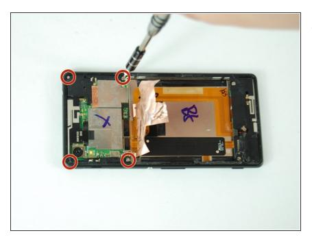
Remove the four hex head 3mm screws at each corner of the motherboard with a screwdriver.
