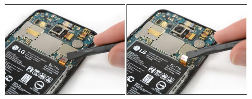
• Use the edge of a spudger to pry up and disconnect the battery flex cable located at the bottom right of the motherboard.
