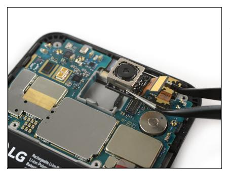
• Use a pair of tweezers to remove the rear facing-camera.
