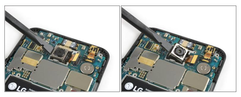
Apply the flat end of a spudger to the left side of the rear-facing camera and carefully lever it out of its recess.
