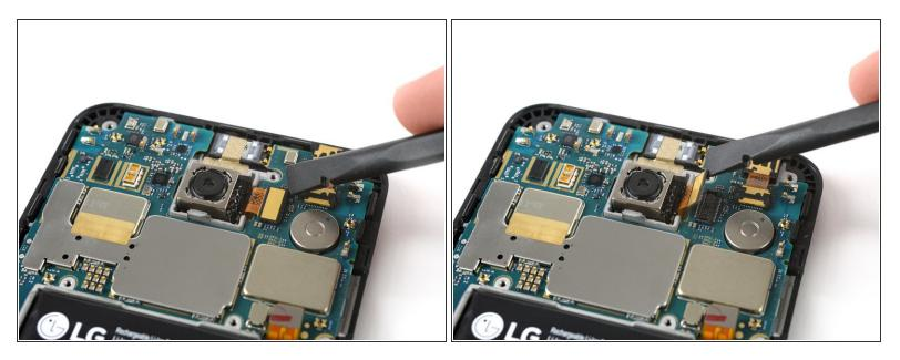
• Use the flat end of a spudger to pry up the rear facing camera's flex connector.
