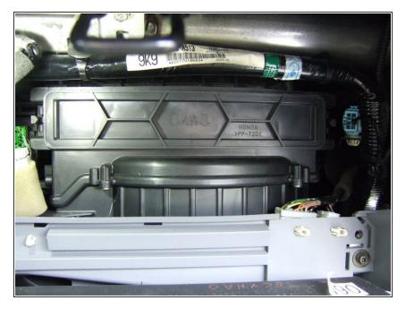
Slide the filter tray back into the heater blower the same way it was removed. The left and right locking tabs should snap into place when it's fully inserted.
