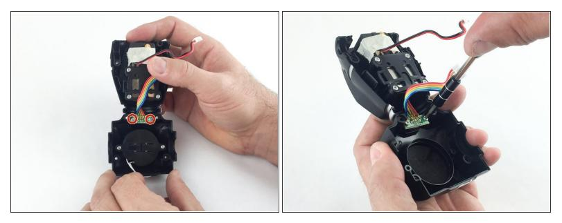
Remove the two 9.3mm Phillips #1 screws.
