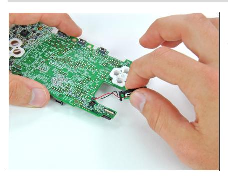
Remove the volume switch from the motherboard. To reassemble your device, follow these instructions in reverse order.
