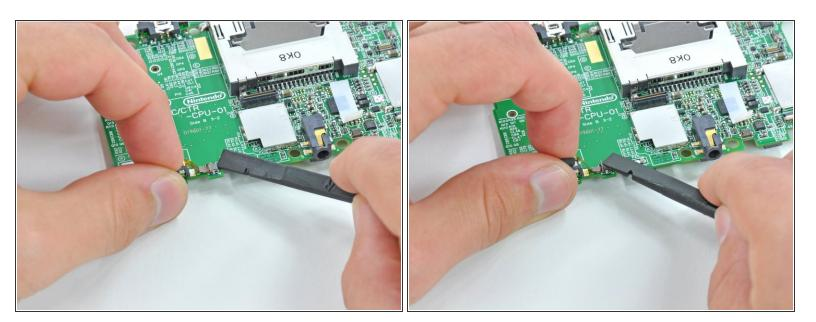
• Use the flat end of a spudger or your fingernail to flip up the retaining flap on the microphone ribbon cable ZIF socket.
