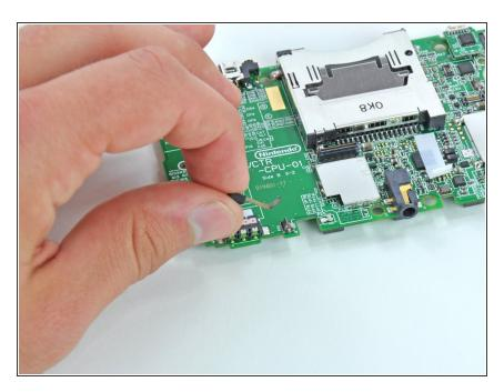
Lift the microphone and its attached ribbon cable off the motherboard. To reassemble your device, follow these instructions in reverse order.
