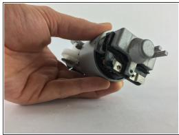
• Firmly grip the motor in your hand. Using pliers, pull the connectors off the motors.
