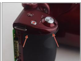
Use the spudger and pry the top cover off starting on the left side and working your way down.
