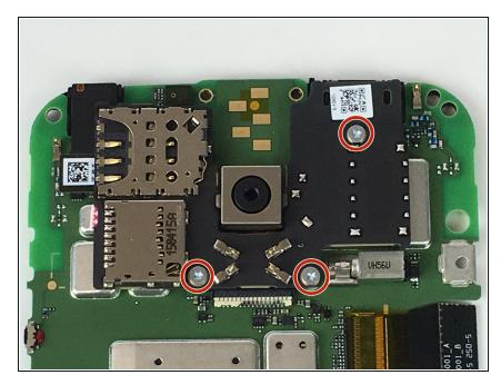
Remove the three 2.4 mm T4 screws from the right side and bottom of the SIM/SD card panel.
