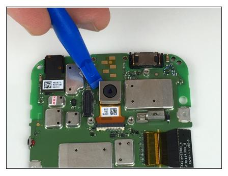
Pry off the main camera from its base using a plastic opening tool.
