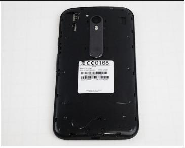
Use your fingernail to pry under the notch on the bottom of the phone and remove the back cover.
