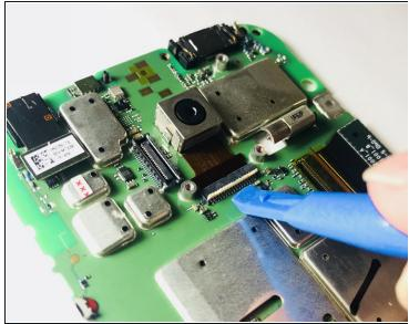
• Use a plastic opening tool to flip up the lock on the camera cable ZIF connector.
