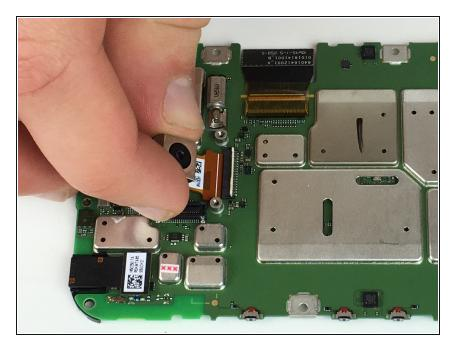
Carefully pull the camera from its socket on the motherboard.
