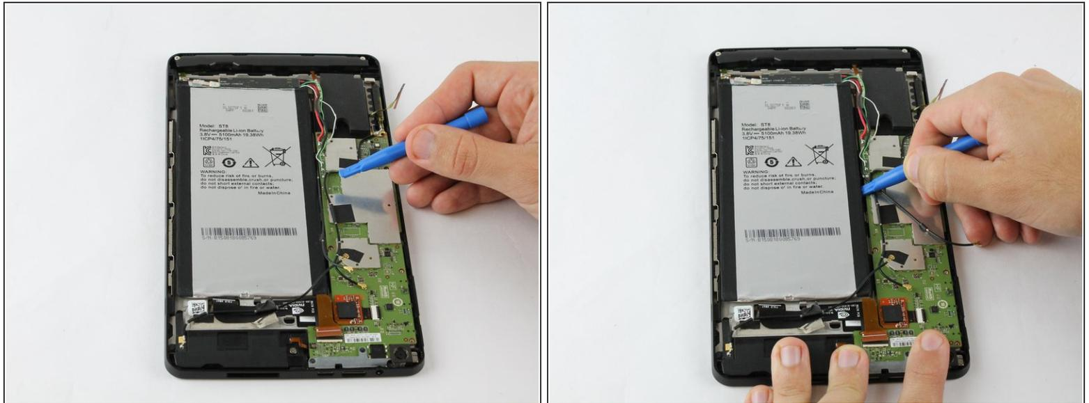
**!** The battery is heavily glued down so you will need to apply force while also exercising caution to not damage the rest of the device.
