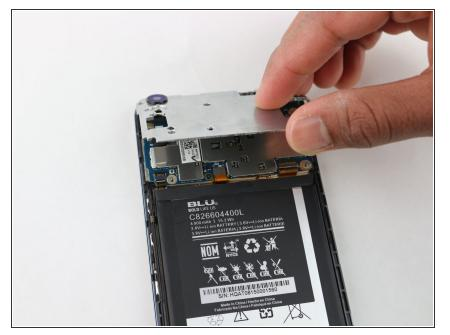
After all the screws are out, lift the protective metal cover off of the phone. Lift from the bottom of the cover.
