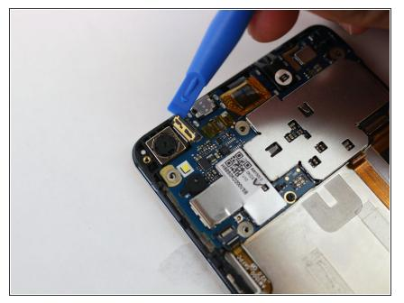
• Loosen the camera from the glue using the small blue plastic opening tool.
