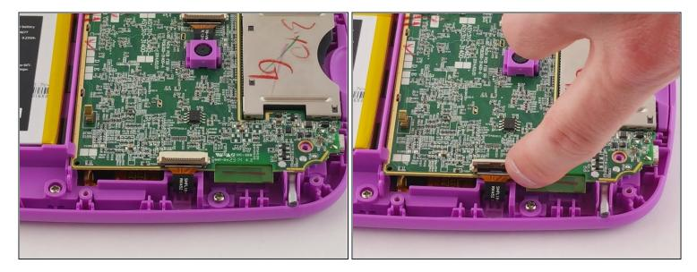
• Unplug the front facing camera cord with an opening tool to free the top of the motherboard.
