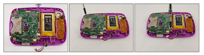
• Remove the three 6 mm phillips head screws holding the motherboard to the display assembly.
