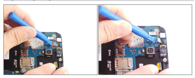
• Use the plastic opening tool to unhook the ribbon cable clip.
