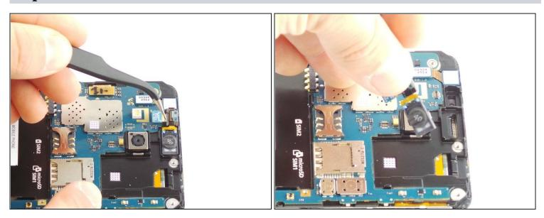
• Gently pull on the connector with the <u>tweezers</u> until the speaker comes off.
