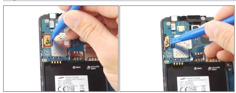
• Unhook the other ribbon cable clip to the screen with the blue plastic opening tool.
