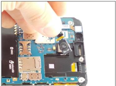
• Gently pull on the connector with the <u>tweezers</u> until the speaker comes off.
