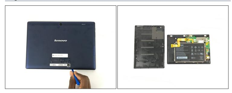
• Use a plastic opening tool to pry open the back cover of the tablet.
