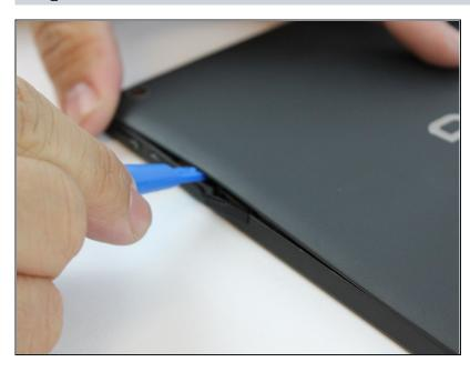
Starting at the Micro SD Card Slot and using the blue plastic opening tool, begin to maneuver the tool around the edges while applying light pressure to lift the panel upwards.
