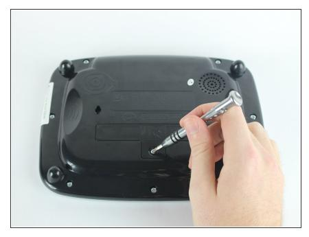
Remove the 9.9 mm screw covering the batteries with a PH1 driver head.
