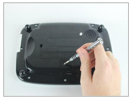
• Remove the 9.9 mm screw covering the batteries with a PH1 driver head.
