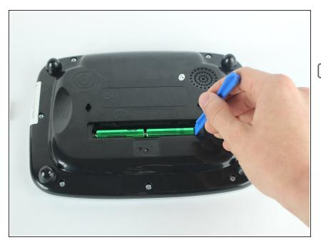
• Use a plastic opening tool to pry the batteries out of their holding.
