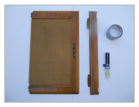
This is the broken dresser drawer, duct tape & 5 minute 2 part wood epoxy.
