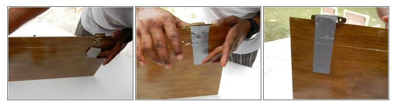
• Attach and align the smaller cabinet door section to the bigger cabinet door section. Press them firmly together and apply the duct tape on both ends for bonding support.
