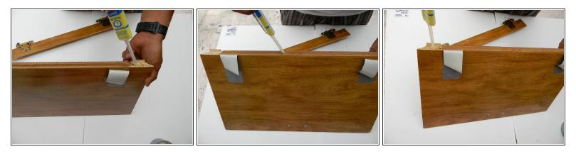
• Run a thick bead of epoxy on the inside rim of the cabinet from one end to the other.
