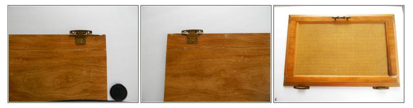
• After at least 15 minutes you can pull tape off completely and wipe away any excess epoxy. It is now finished and ready to be re-installed back to the cabinet.
