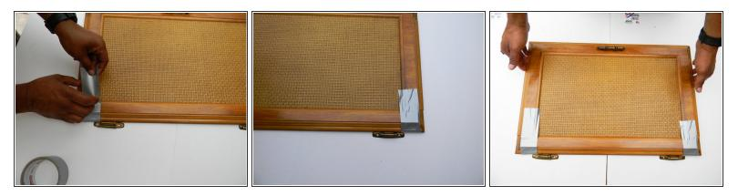
• Flip door over to front side and tape both ends of the cabinet. This will add more support while it is drying.
