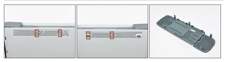
(i) In the next few steps, you will use the tip of a spudger or the finger of an Xbox 360 opening tool to release the clips along the left and right sides of the top vent. Their locations are highlighted in red.
