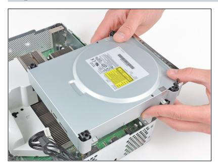
• Lift the optical drive assembly out of the metal casing.
