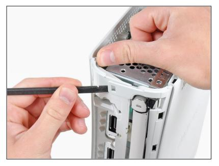
• Insert the flat end of a spudger and pry upwards to release the last remaining latch located above the eject button.
