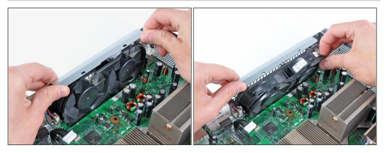
• While lifting the metal chassis strip above the dual fans, pull the fans toward the center of the motherboard.
