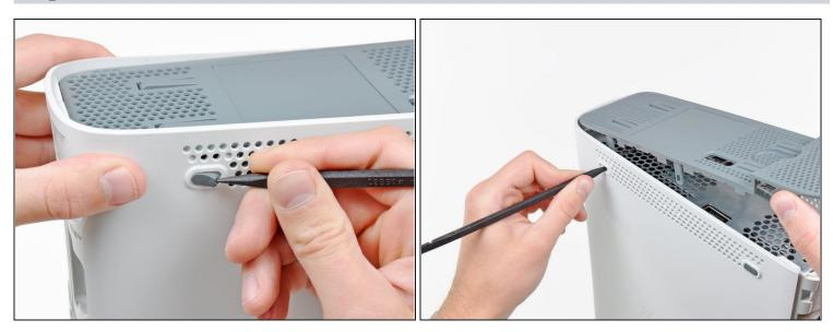
(*i*) The last clip is hidden underneath the rubber foot nearest the back of the console.
