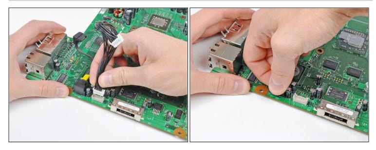
• Disconnect the optical drive power and SATA cables from the motherboard.
