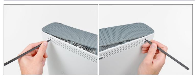
• Use the tip of your spudger to release the clips on the bottom vent nearest the back of the Xbox.
