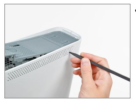
• Use the tip of your spudger to release the clip on the top vent nearest the back of the Xbox's upper case.
