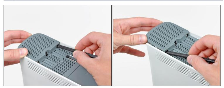
• Insert the flat end of a spudger into the small gaps previously mentioned to release the clips.
