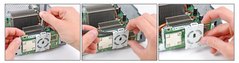
• Use the flat end of a spudger to release the clips securing the RF module shield along the top and the left edge of the RF module.
