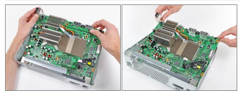
(i) Turn the Xbox over, being careful not to let the motherboard fall out of the chassis.
