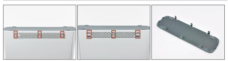
(i) In the next few steps, you will use the tip of a spudger or the finger of an Xbox 360 opening tool to release the clips along the left and right sides of the bottom vent. Their locations are highlighted in red.
