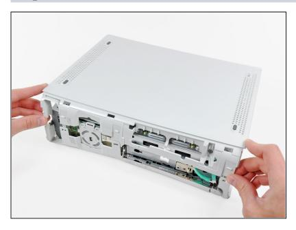
• Slightly lift the front portion of the lower case to ensure that the latches in the front have been completely released.
