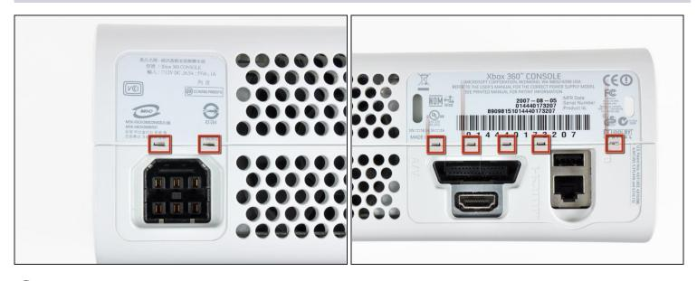
(i) The upper and lower cases are held together by seven release latches located on the back of the console. Their locations are highlighted in red.
