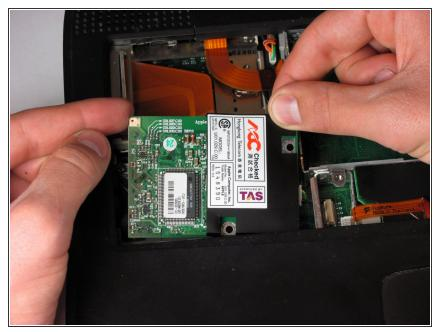
• Using your fingers, lift the modem from the socket it is plugged into.
