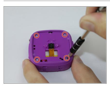
Unscrew the (4) 2.5mm Phillips head screws from the third layer of plating using a #0 screwdriver.
