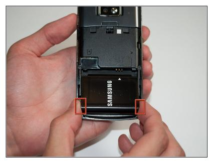
Grasp the bottom corners of the battery with two fingers and gently lift.
