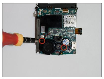
Using a Phillips #00 screwdriver, unscrew the two 3.5mm screws that connect the speaker to the motherboard.
