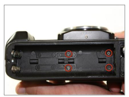
Use a 00 Phillips head screwdriver to remove the four screws from inside the case.
