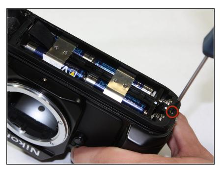
Use a 00 Phillips head screwdriver to remove the small screw on the far left of the battery compartment.
