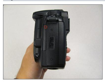
Remove the 4.8 mm black screw on the left side of the camera.
