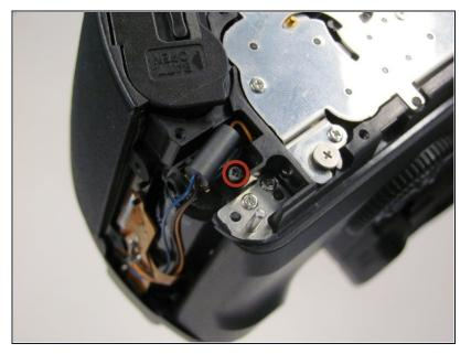
• Remove the single 4.8 silver screw from the control socket.
