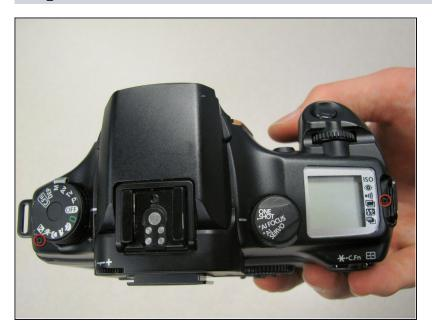
Remove the two 4.75 mm black screws located on the top of the camera.
