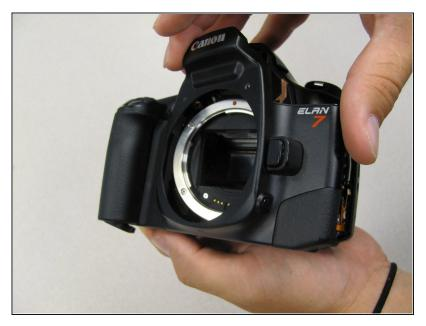
Remove the front panel by lifting it away from the camera's body.
