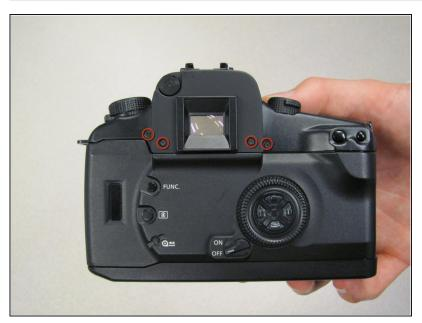
• Remove the four 4.3 mm black screws near the bottom corners of the eyepiece at the back of the camera.
