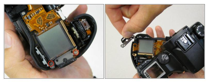
Remove one 8.5 mm silver screw (front) and one 5.45 mm silver screw (back) to remove strap loop near LCD screen.
