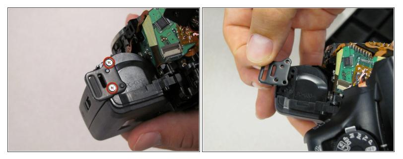
• Remove two 5.9 mm silver screws on top of camera to detach left strap loop (opposite grip).
