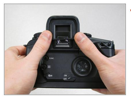
Slide the outer eyepiece upward to remove it.
