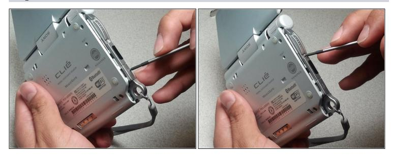
• Gently pry rear cover to remove USB port cover and Hold Switch.
