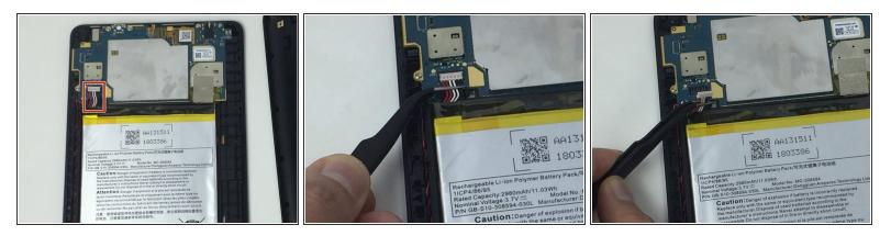
Using angled ESD precision tweezers, lift up on the battery cables to separate the battery connector from its socket.
